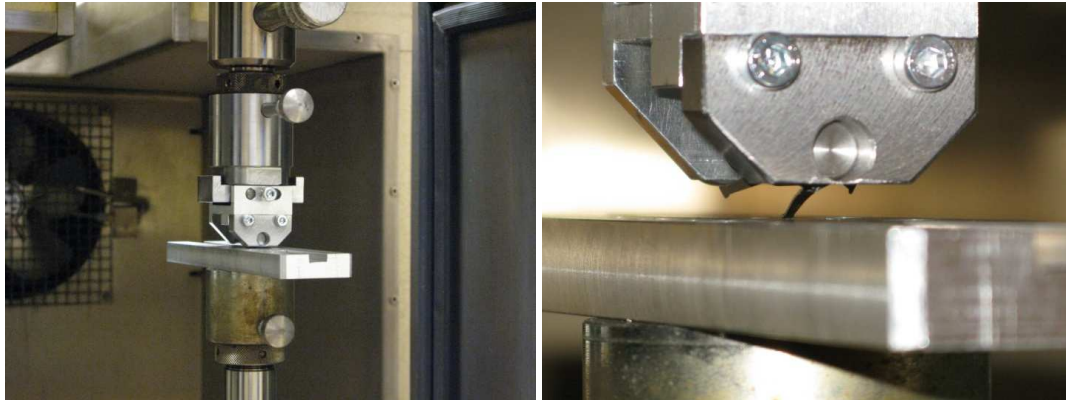
Figure 5: Experimental device made for testing the prongs
